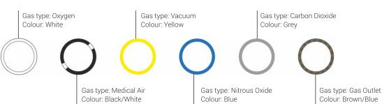
**Application:** Reinforced tubing for gas supply **Material:** Inner layer: Antistatic Polyurethane. Outer layers: food grade PVC, DEHP free, 80 Shore **Structure:** 4-layer hose reinforced with polyester yarn
