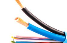
Material: PVC Structure: 1-layer non-reinforced hose Colour: Several colours available. Also with a stripe Inner diameter (mm): 1-60 Lengths depending on size (m): 50-5000
